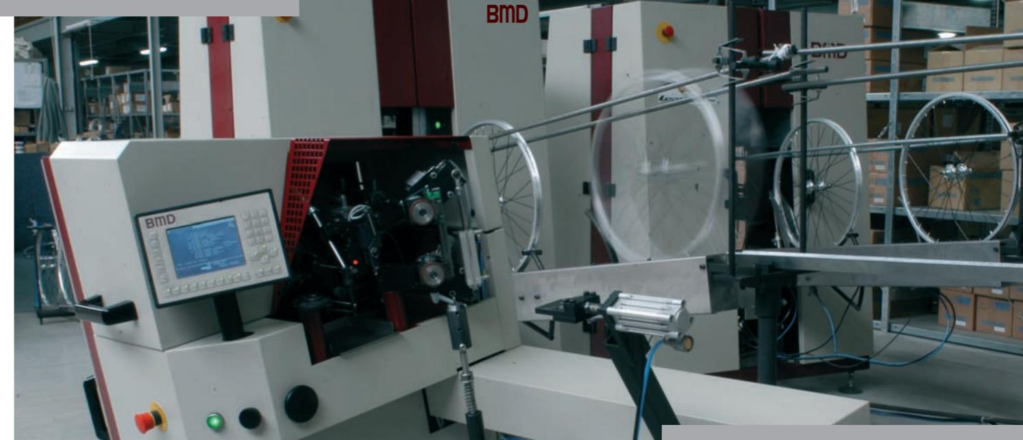
The CC lacing machine, combines in one machine lacing and tightening according to a well-tried method. Standard it works with extremely high rims up to 45 mm from 16" to 28". It standard handles all special lacing patterns, as it is standard. To provide an ergonomic working position for different operators the working height of the machine is adjustable over a range of 200 mm and is placed at a slight angle.
